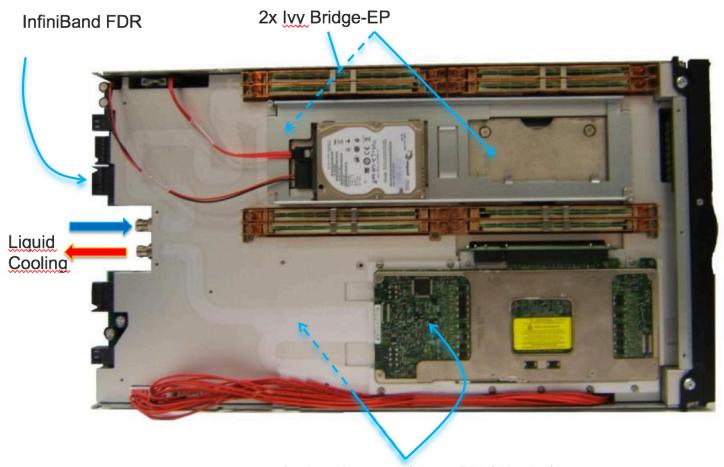
2x Accelerators (Xeon Phi / Kepler)
